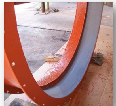
mClad ™ mFill ™ restores the flange face for a proper seal
