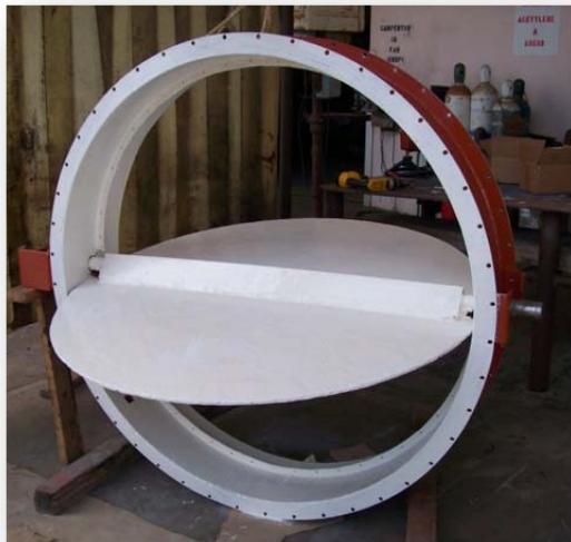
Two coats of MCOR ™ 2101 ensure ceramic protection against further corrosion and chemical attack
