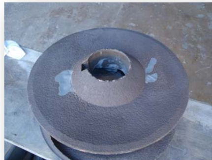
MCOR ™ 3310 was then used to reclaim
